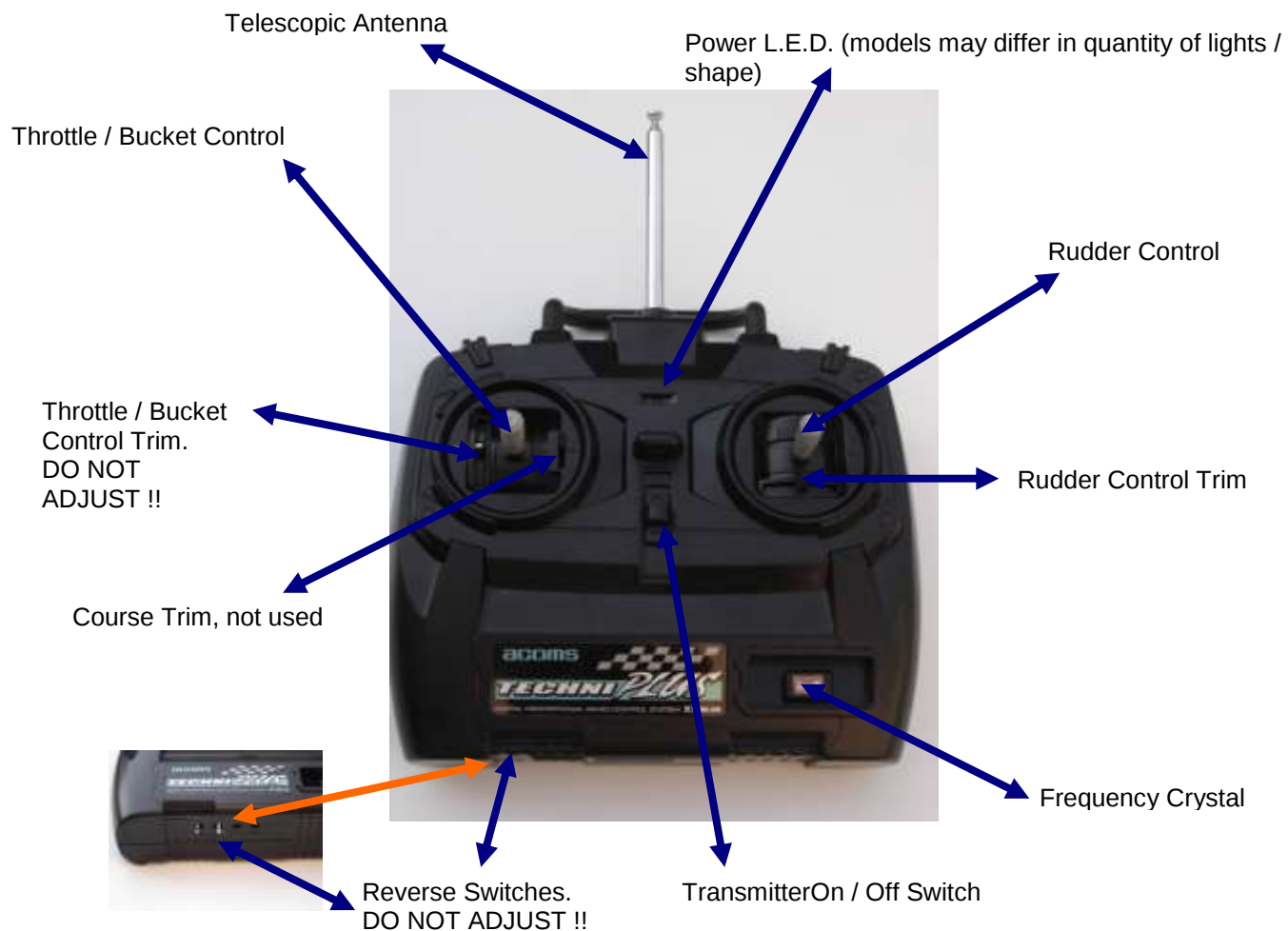
Figure 3: Layout of Transmitter Radio (some models may vary)
